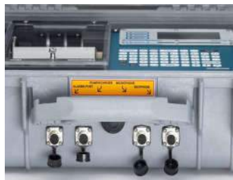
Instrument connection ports come standard with caps to protect connecting pins.
